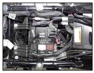
**FL-K:** Connect the oxygen sensor harnesses to the AutoTune harness, you will hear a click when they are connected properly. Carefully wire tie the leads to the motorcycle. Take extra care to ensure harness and sensor leads are safe from rubbing or chaffing on the motorcycle. Use all supplied wire ties; add extra ties if needed to properly secure wiring on your installation.
