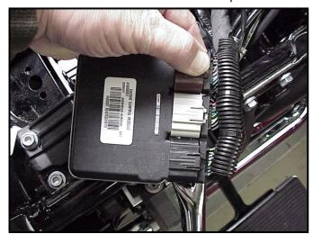
**FL-G:** With the factory ECM removed, route the AutoTune harness thru the opening on right side of the frame below the down tube for the seat, towards the ECM caddy.
