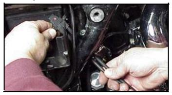
**FL-H:**. Route the AutoTune harness plug under the brake lines to the ECM caddy area. Locate the package of dielectric grease included with communication cable. Spread a small amount of grease on the AutoTune harness plug end and inboard of the mounting flange to allow the plug to easily slide into the ThunderMax ECM. Install in case with the ThunderMax logo up and attach with the provided screws.
