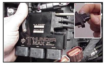
**FL-I:** Install main harness connectors to ThunderMax ECM. Before installing the connectors, lightly spread some dielectric grease on harness connector terminals.
